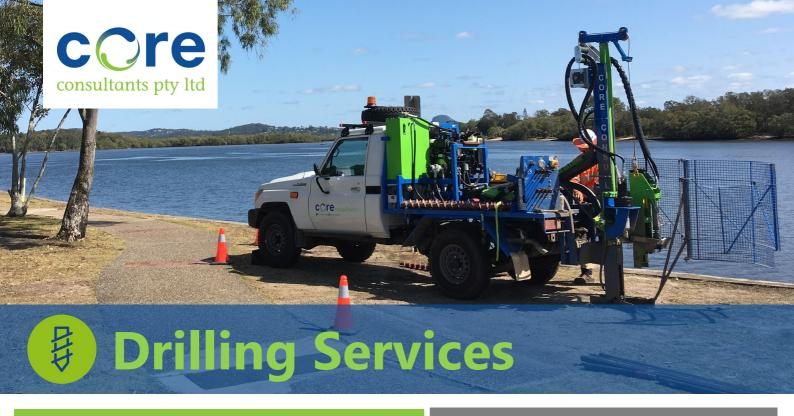
Core Consultants' drill rig is custom-built for geotechnical and environmental investigations
